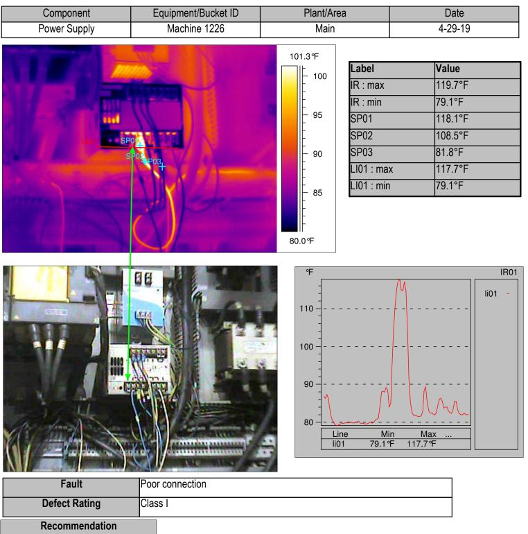
Localized hot spot indicates poor connection at wire terminal. Inspect and tighten connection if possible. Replace as necessary.
