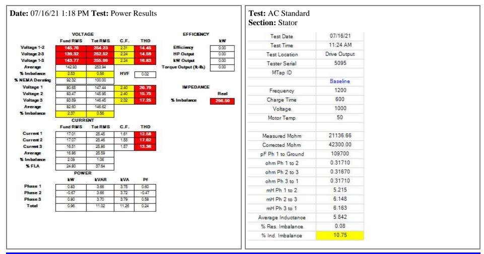
Remarks:The off line data indicates that the motor has some inductive imbalance of 10.75%. some motors can run as high as 17%. i see this as no issue for now.
