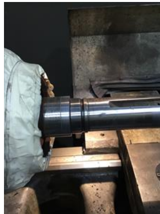
Welded and remachined bearing fit
