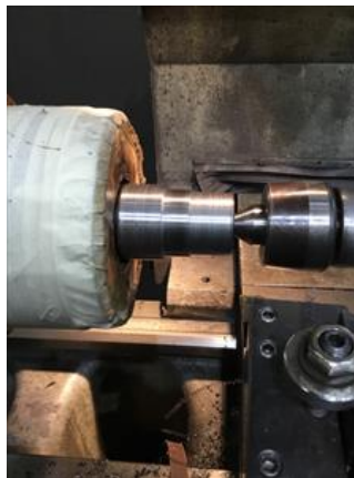
Welded and machined fits
