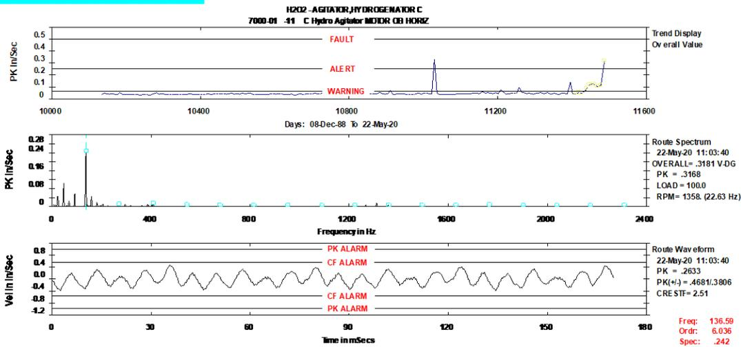
**NOTE: There is a small gearbox lubrication pump adjacent to the motor that could be affecting the vibration seen in the motor and gearbox that is not on our vibration route. This unit should be inspected soon.**
