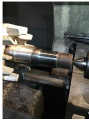
After Shaft at Bearing cap- 2.490 Shaft at endbell- 2.046
