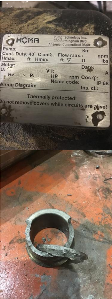
Drive end bearing race cracked
