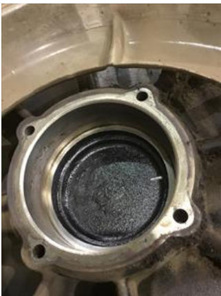
Bearing slid off of shaft with end bell revealing bad fit
