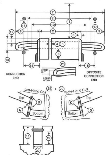
High Speed winding data 6 groups of 4 44 T/C 1#22 Wire 1 & 11 Span 1Y Connection 12" SAB Leads #11,12,13 Used 9.0 Lbs. 1#22
