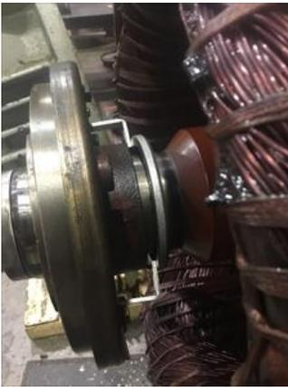
25. Drive End Wavy Washer/Snap-Ring Other Retention Device?
