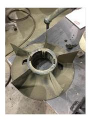
34. Broken or missing components Fan blade lock tabs broken.
