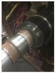
58.Lubrication Typepink grease59.Grease Condition(F) FailP74
