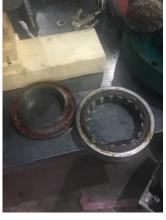
Bearing DE Type roller and ball 52. 53. DE Bearing Qty. 2
