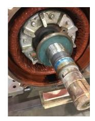
55. Bearing ODE Type regular ball bearing P53
