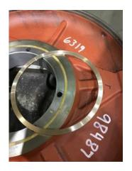
.195 spacer to lock bearing in place.
