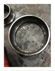
52. Bearing DE Type P23 Thrust ball bearing
