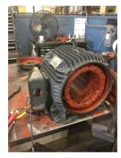
Fan Condition (P) Pass 34. Broken or missing components **Initial Electric Test** 0 35. Resistance to Ground Winding Resistance 1-2 36. 37. Winding Resistance 2-3 38. Winding Resistance 1-3 39. Resistive Imbalance 40. Hi-Pot P58 41. Surge Test (P) Pass
