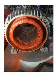
43. Failure Location ode housing fit **Initial Rotor Inspection** 0 44. Rotor Type squirrel cage laminate 45. Air Gap <10% Variation 46. Number of Rotor Bars 47. Number of Broken Rotor Bars **Growler Test** 48. (P) Pass P50 **Rotor Condition** 49.
