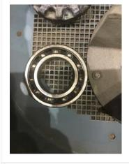
55. Bearing ODE Type regular ball bearing
