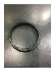
65. ODE Seal Type/Size dust shield **Root Cause of Failure** bearings 66. Component Failure 67. Cause of Failure Bearings over greased/grease contaminated/dirty. 68. Comments
