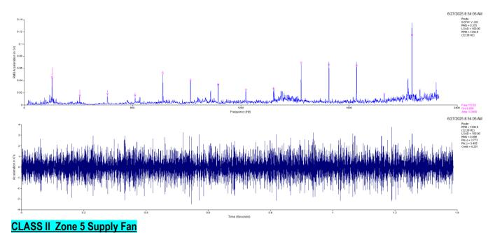
Fan inboard (DE) bearing data shows non-synchronous harmonics in the spectrum. This is an indication of bearing defects. Inspect fan bearings for defects and wear as scheduling allows.
