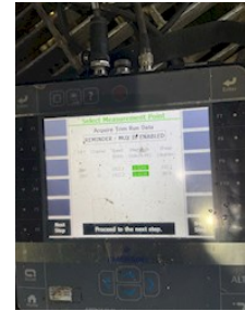
Jet drier 1 nozzle fan is good after balancing. Needed cleaned and balanced.
