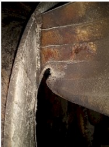
Preheat aspiration fan blades have a lot of wear on them.
