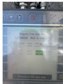
Flakes aspiration fan. Started at 1.9 and 1.7. Ended at 0.3 and 0.6. Needed cleaned
