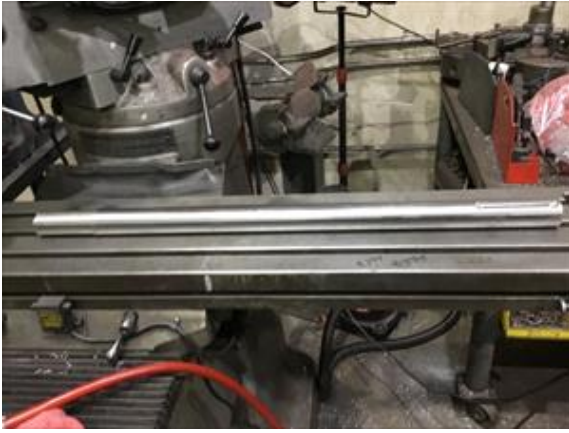
Machined new shaft GM
