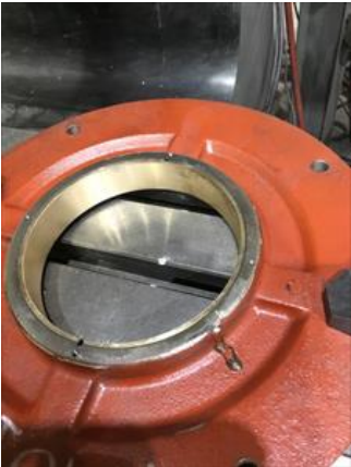
Sleeved bearing inner bearing cap. Clearance- .030"
