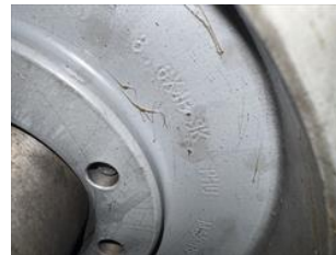
Ah10 supply fan pulley. 8.6x4B SK PHU
