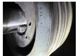
Ah11 return motor pulley. 7.0x3B SK TID
