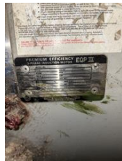
8 return 2. Motor bearings are 6310ZC3 and 6310
