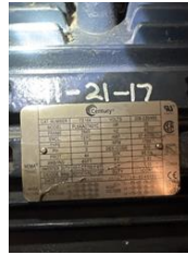
Ah11 return Motor bearings are 6311c3 and 6210c3
