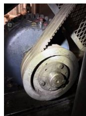
Ah11 return motor pulley 7" diameter shaft 1 7/8"
