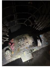
8 supply ODE 2.6875 shaft. Link Belt bearing with no data
