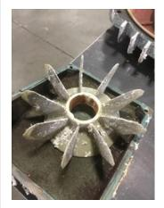
Fan saw excessive heat from bearing failure and cracked.
