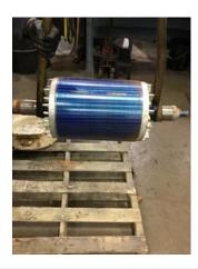
51. List the Parts needed for the Repair Below 6313 ZZ C3 6213 ZZ C3
