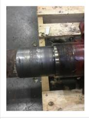
55. Drive End Bearing Shaft Fit Condition
