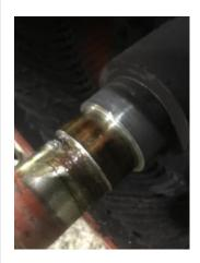
57. Opposite Drive End Bearing Shaft Fit Condition(P) Pass
