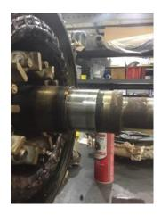
55. Drive End Bearing Shaft Fit Condition
