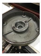
87. Bearing Cap Condition Post Repair
