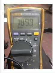
28. Stator Overloads/Ohms
