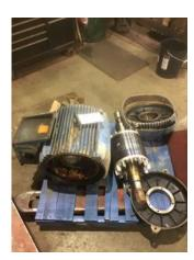
Describe the Overall Condition of the Equipment as Received Serviceable (No) No Is this a UL Listed Motor 6. Is the motor water cooled or can be pressure checked before teardown (No) No Initial Mechanical/Electrical 0 (Y) Yes 7. Does Shaft Turn Freely? 8. Does the shaft require T.I.R in Lathe to identify additional repairs? (No) No Does Shaft Have Visible Damage? (No) No 9. 0.001 Inches 10. Assembled Shaft Runout Assembled Shaft End Play 0 inches 11. Air Gap Variation <10%
