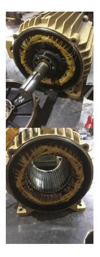
Describe the Overall Condition of the Equipment as Received Is this a UL Listed Motor (No) No 5. Is the motor water cooled or can be pressure checked before teardown (No) No Initial Mechanical/Electrical 0 7. Does Shaft Turn Freely? (Y) Yes 8. Does the shaft require T.I.R in Lathe to identify additional repairs? (No) No Does Shaft Have Visible Damage? (No) No 9. Assembled Shaft Runout 0.001 Inches 10. 11. Assembled Shaft End Play inches 12. Air Gap Variation <10%
