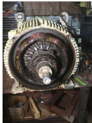
ODE bearing cap bolts loose. (All of them.)
