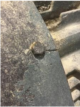
Small crack in fan cover mount bolt hole
