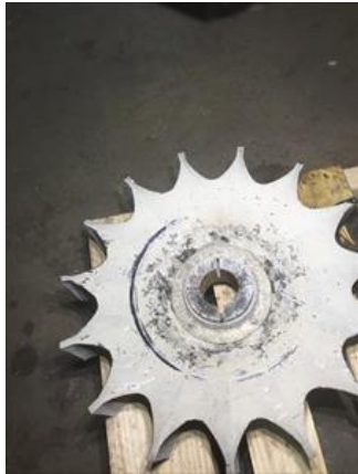
Some wear from loose bearing cap bolts
