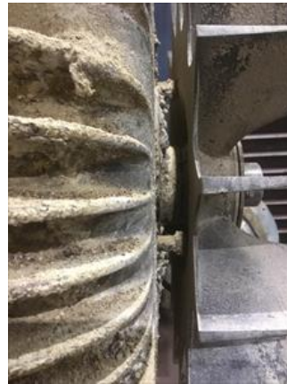
ODE bearing cap bolts loose. (All of them.)
