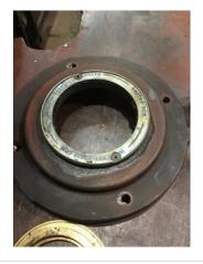
32. Drive End Wavy Washer/Snap-Ring Other Retention Device?
