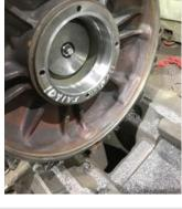
90. Opposite Drive End - Endbell Bearing Fit Post Repair 0 Degrees 60 Degrees 120 Degrees
