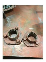
64. End Bell Air Seal Fits Opposite Drive End Air Seal Drive End Air Seal
