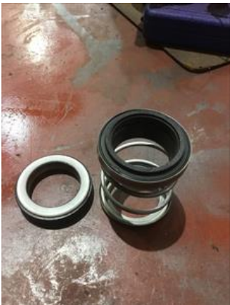
Inner seal OD: 1.8825 Shaft diameter: 1.2502
