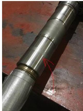
Outer seal surface has wear.
