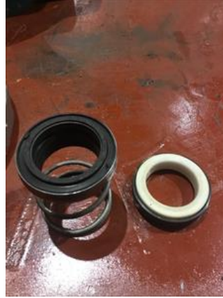
Outer seal O.D 1.7560 Shaft diameter: 1.1255 Carbon ceramic
