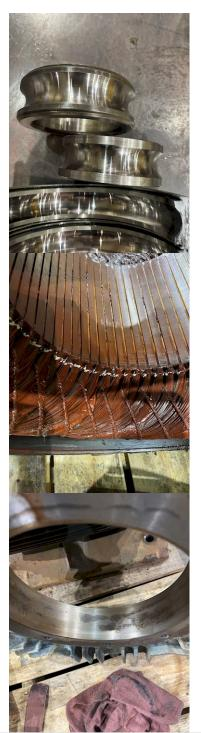
4. Describe the Overall Condition of the Equipment as Received Windings are shorted. Needs rewind and bearings.
