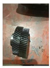
Describe the Overall Condition of the Equipment as Received Rotors locked up and rusted.
