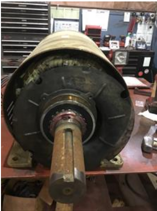
Missing mount bolt
