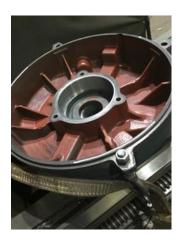
82. Bearing Cap Condition Post Repair
