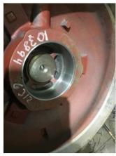
75. Bearing Cap Condition Post Repair
