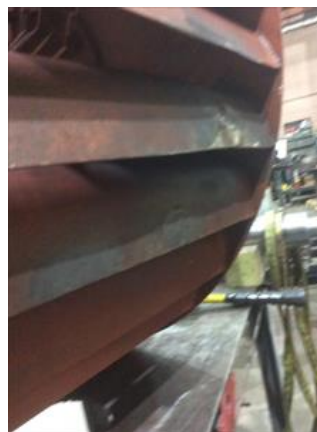
Repaired bent blades.
