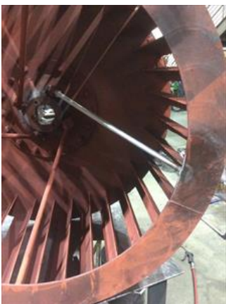
Replaced broken support bar.
