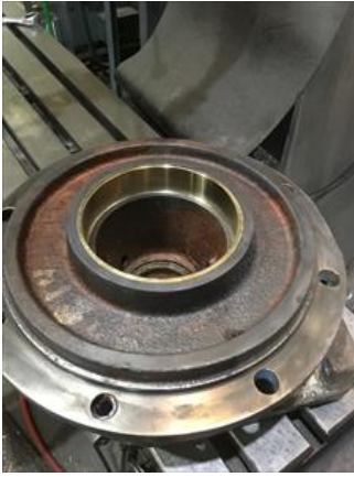
Installed upper wear ring. Clearance .03"
