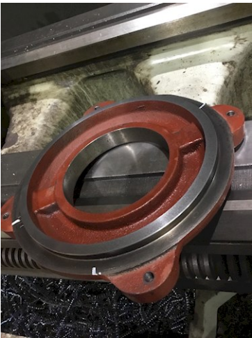
Reduced O.D.E. bearing cap shoulder by .06 and increased housing depth by .06 for thermal expansion. Changed locked bearing from O.D.E. to D.E.
