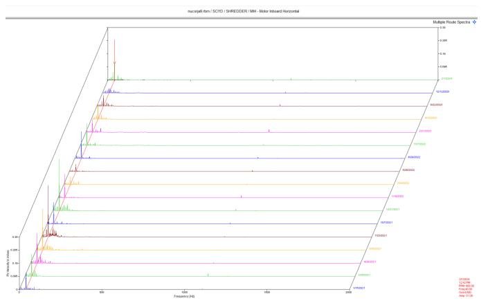
This vibration is on the lower side compared to historical data. Amplitude is well below alarm level. .3 ips is where the first alarm level is set at. 1 x rpm vibration is very low. If there was imbalance in the motor or index gear, 1x rpm amplitude would be high. Recent data shows 1 x rpm vibration to be below .1 ips which is well within specifications of a 600 rpm motor. No issues to note at this time.
