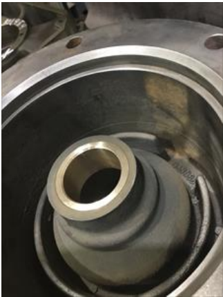
Machined new bushing. 1.506 Gary
