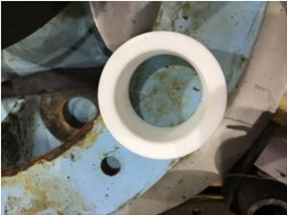
Machined new shaft bushing.
