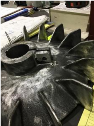
Repaired broken fan. Gary
