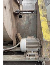
Small fan could not get small fan below 4 mils, suggest checking bearings to see if they are showing signs of wear
