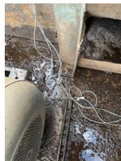
West side of East side fan has all mounting hardware broken off. Due to that I couldn't get it under 5 mils
