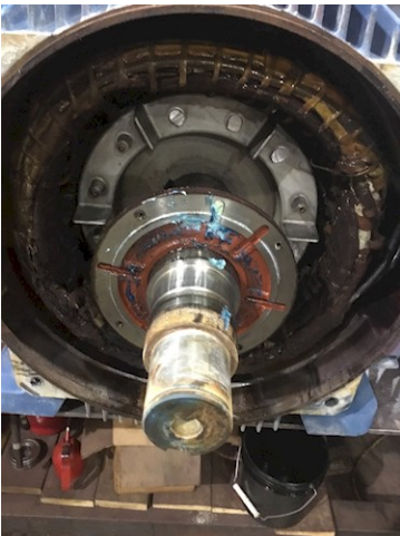
Has a water line almost half way up the windings
