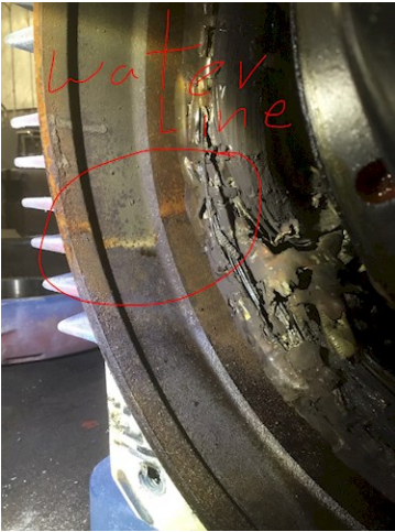
Has a water line almost half way up the windings
